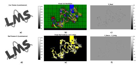
**Figure 2:** Example HEVC/H.265 encoding of a rotating frame (a) with LowDelayP and QP=20. All information was exported by HARP during runtime, creating a POC object, which can then be imported, analyzed and visualized in Python (b-f). Same is true for all following figures.
