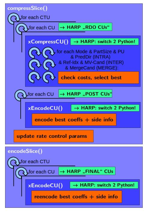
**Figure 1:** Outline of basic HM encoder architecture. HARP natively attaches to the HM encoder and provides detailed insight (green).
