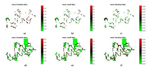
**Figure 4:** Analysis of HEVC/H.265 coefficient / side information bits for the rotating frame depicted in Fig. 2. Here, only POST-CUs were used for visualization. Top row shows intra modes, bottom row inter modes. Note the high number of bits required for transmitting the coefficients (center).
