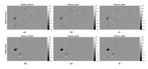
Figure 5: Analysis of residuals after HEVC/H.265 conducted 2Nx2N, Nx2N and 2NxN RDO inter checks for the rotating frame depicted in Fig. 2. For clarity, only depth 1 and 3 are shown, with the best MV and Refldx found.
